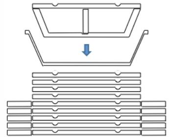
Polar DotBox™ is stackable, modular and can be pressure washed. Several different configurations are available and all are interchangeable.
